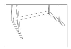
Attach the Base Plate to the Welded Side Uprights using (2) 5/16" x 3/4" Flat Head Machine Screws, 5/16" Lock Washers, and 5/16" Hex Nuts. **HAND TIGHTEN ONLY.**
